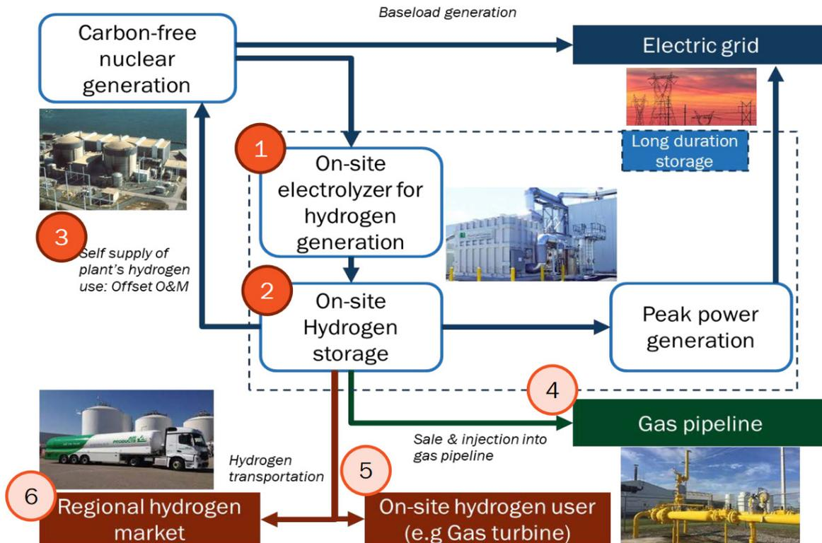
Fig. 8 - Example of a demonstration project within the US: Repurposing Nuclear Plants using Hybrid Hydrogen Approach<sup>35</sup>
