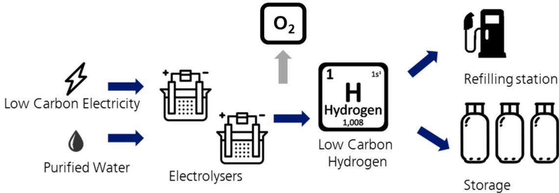
Fig. 6 - Electrolysis basic components and process<sup>28</sup>
